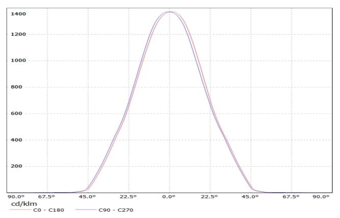
NOTE: The typical divergence will be changed by different color, chip size and chip position tolerance. The typical total divergence is the full angle measured where the luminous intensity is half of the peak value.
